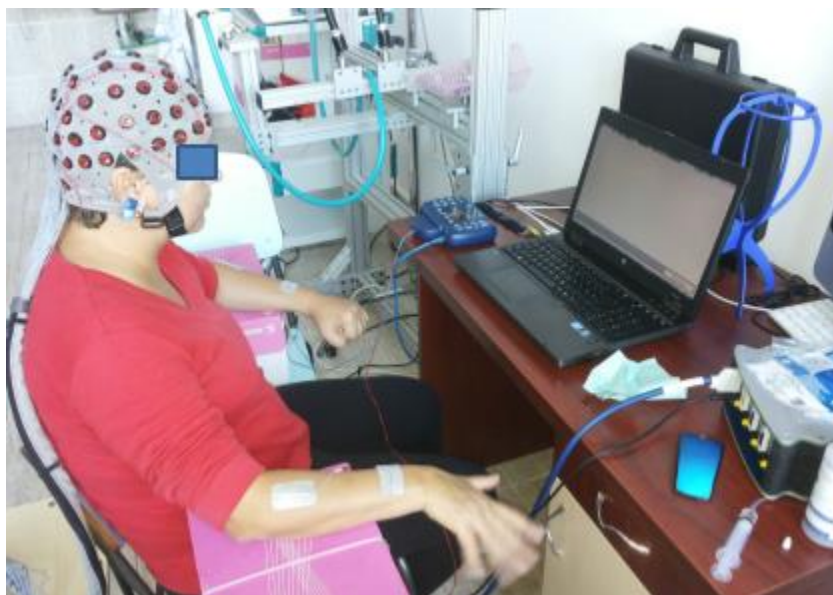
Figure 2 – The BCI&FES upper limb rehabilitation RecoveriX system (Rehabilitation Hospital of Iasi clinical tests)
